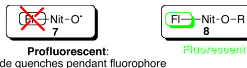
Figure 2. Profluorescent nitroxides 7: the free nitroxide quenches fluorescence of a closely tethered fluorophore; fluorescence is restored upon reaction to form the N -alkoxyamine 8.
